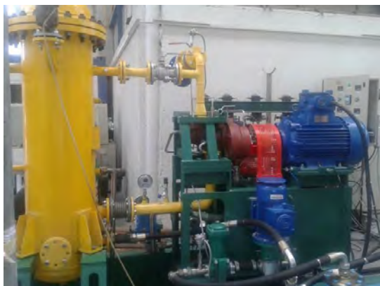
Fig. 1. Expander on the COMOTI's test bench
