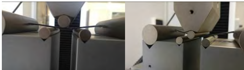
Fig. 5 Samples subjected to 3-point bend tests [11]
