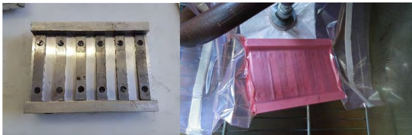
Fig. 4 Multi-nest mould and the vacuum bag assembly for sample fabrication [11]
